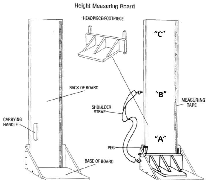
is positioned. Hold the sliding head/footpiece by the center triangle and slide it the length of the assembled board to make sure it is functioning properly.
