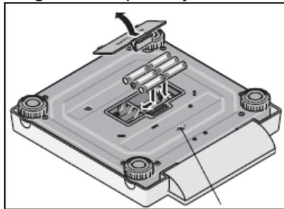
3. **Setting up and aligning the scale:** If the surface is not level, align the scale by turning the foot screws. The air bubble in the spirit level must be in the center of the circle. Ensure that only the feet of the scale are in contact with the floor. The scale itself may not be in contact with the hard surface at any point. The alignment of the base of the scale must be checked and corrected as necessary every time the location of the scale is changed.
